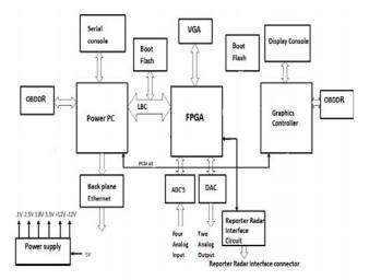
Figure 3: Simulator Hardware Architecture
