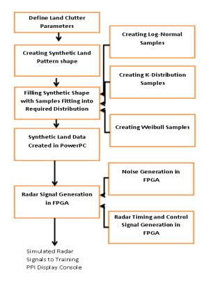
Figure 4: Simulator Algorithm and Signal Flow Chart
